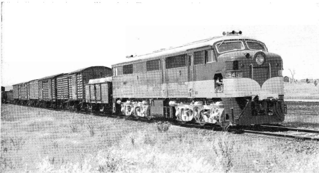
NEW South Australian diesel-electric locomotive 945 passes through Victoria on its way from Sydney—at the head of a goods train to Adelaide. Its bogies had been changed at Bandiana from 4' 8½" to 5' 3" gauge.
