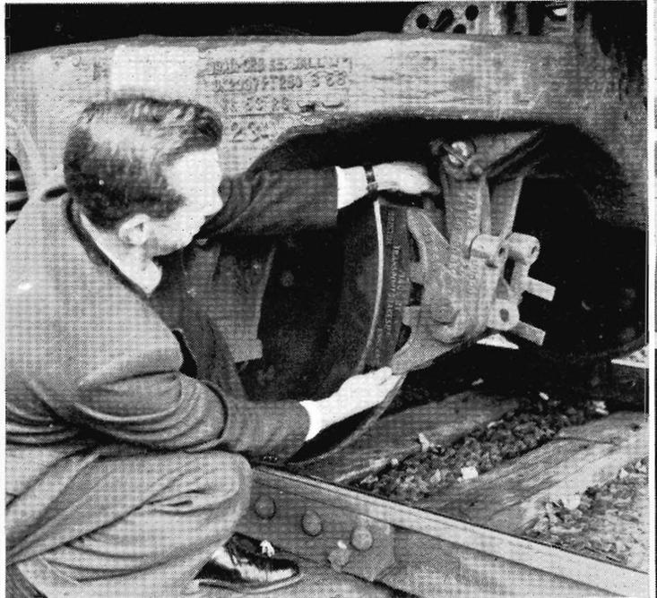
(Above) TESTS are being made with a new type composition brake-block for Harris Trains. Aim is to establish its length of life and train-stopping capabilities, with noise and maintenance-cost reductions. (Right) On the 30 new Harris Trains, it will be possible to open and close each door individually; on those now in running both doors move simultaneously.
