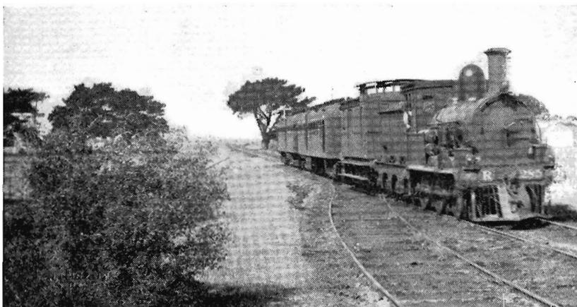
BEFORE electrification many old steam locomotives had their last working days on the Altona line. R-class 0-6-0 No. 285 is seen here hauling the Altona train: a Z van and two motorless McKeen cars. (Photo.: W. H. Ellis collection).
