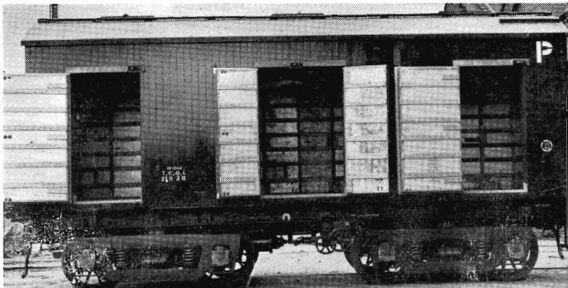
FITTED with passenger-type bogies for service on the Mildura Fruit Flier, as well as passenger trains, this specially adapted insulated van has three independently iced compartments for carrying up to 15 tons of varied perishables.
